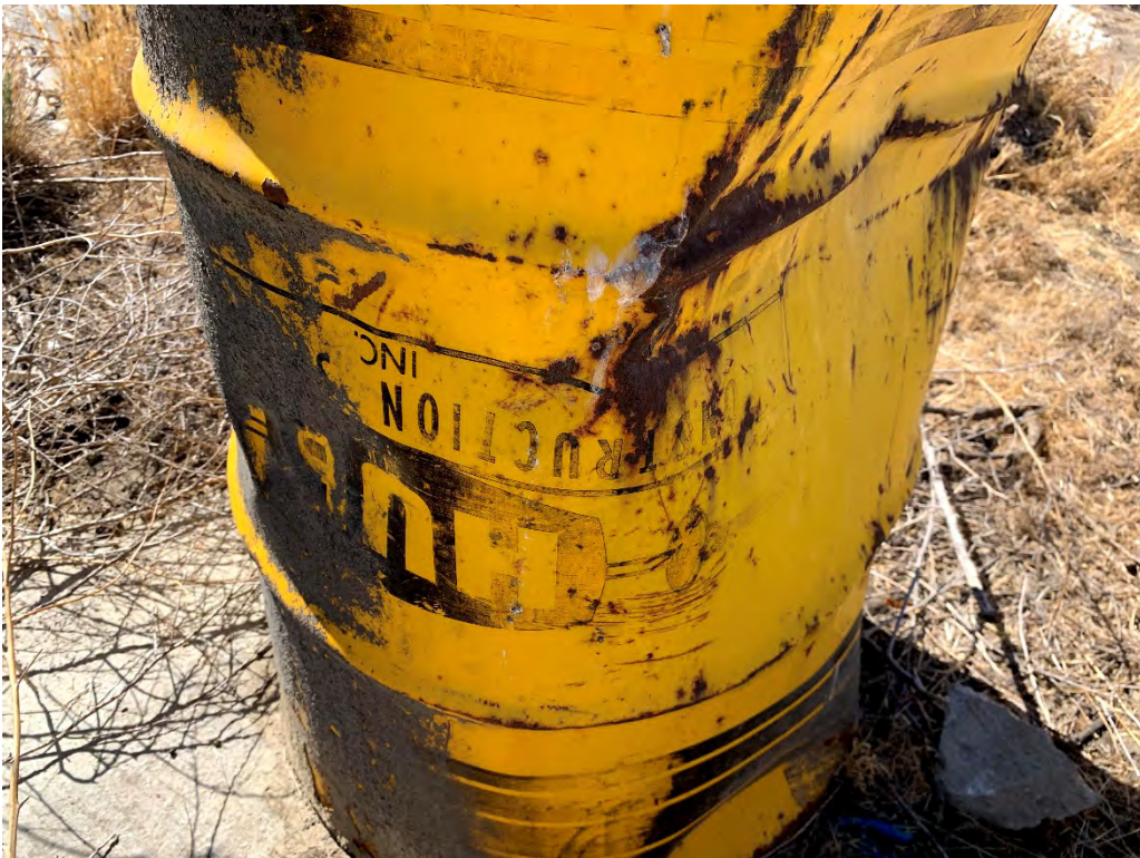
G-6. Exterior of abandoned, un-labeled drum. The surface was damaged and the top lid (bottom) was missing (08/03/2021).
