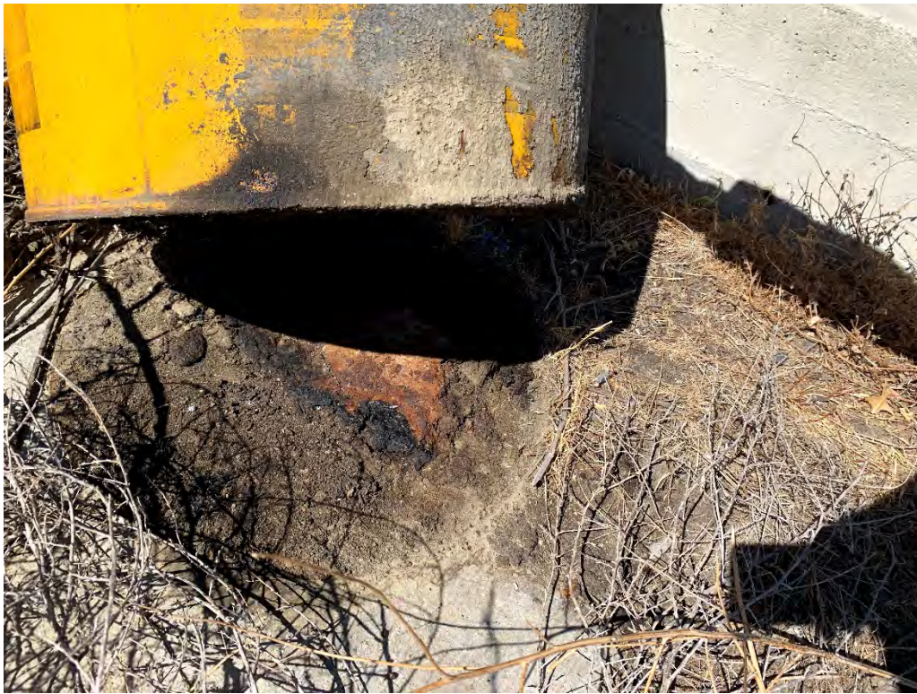
G-7. Caking and potential staining underneath abandoned drum (08/03/2021).
